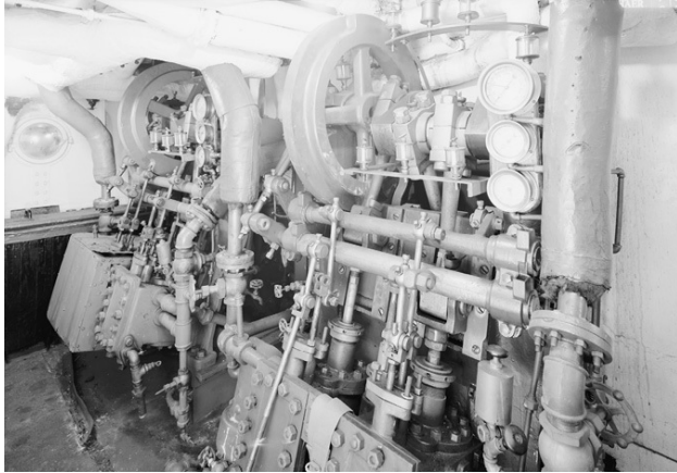
Figure 7.5. Steam-powered refrigeration compressor or ice machine on USS Olympia . Reproduction Number: HAER PA,51-PHILA,714—40 in Collection: Historic American Buildings Survey/Historic American Engineering Record/Historic American Landscapes Survey . Courtesy of Library of Congress Digital Collections. http://www.loc.gov/pictures/item/pa3529.photos.360742p/ .
